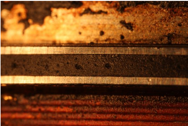
OEM 2pc Ring – Oil Drain Holes Clogged
