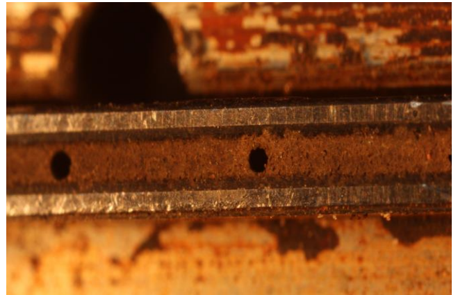
OEM 2pc Ring – Oil Drain Holes Cleaned
